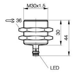
Inductive Sensors BES 516-327-G-E5-Y-S 49 M30x1.5 x 44 normally-open Sn=15mm shielded
